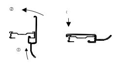
To install the handle, place handle to bottom rail. Flip over and snap into the groove of the rail. To remove handle, hold the bottom rail, detach handle from rail and flip over.
